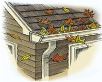
Gutters also need to be wide enough to catch the water when it is raging off your roof during a downpour. When Lakeshore switched from cedar to concrete roof tiles the new tiles extended further out from the roof. The distance from the edge of the roof tile is now often insufficient to allow rain water to enter the gutter and it just flies airborne over the gutter and onto whatever lies below. The solution is a wider gutter, typically a six inch wide gutter.
